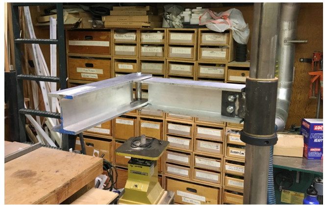
Prototype of arm built by the scenic carpenters to test structure and engineering for movement
