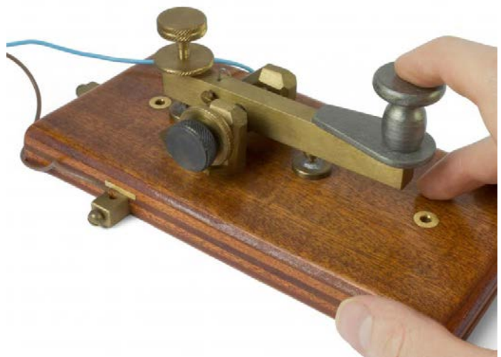
To send messages in Morse code, telegraph operators tapped the knob on a telegraph key.
